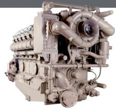
The V228 IMO II emissions compliant engine series delivers a continuous power range from 1,961 bkW at 900 rpm to 3,051 bkW at 1050 rpm (2,630 bhp to 4,091 bhp) for marine applications. Our easy to service unitized cylinder assembly concept enables quick change outs for increased engine uptime. A high capacity turbocharger, electronic fuel injection and efficient combustion management by our engine controller make fuel and lube-oil consumption among the lowest in the industry.
