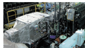
SCR system installation on test bench
