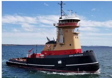
REINAUER TRANSPORTATION M.V. Bert Reinauer 2 x GE 12V250MDC (Mechanical Propulsion) Articulated Tug Barge (ATB)
