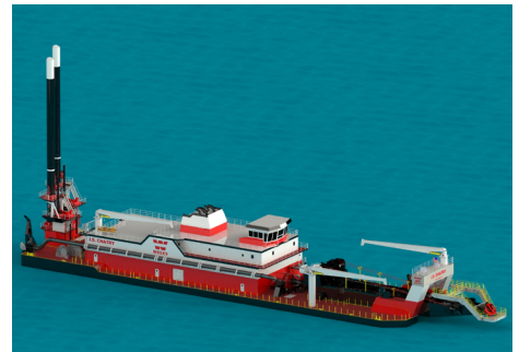
WEEKS MARINE J.S. Chatry 2 x GE 16V250MDC and 3 x 8L250MDC (Mechanical Pump Drive and Diesel Electric Power) Cutter Head Dredging Vessel
