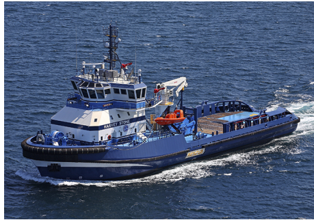
HARVEY GULF M.V. Harvey Stone 2 x GE 12V250MDC (Diesel Electric Power and Propulsion) Multi-Purpose Field Support Vessel (MPFSV)
