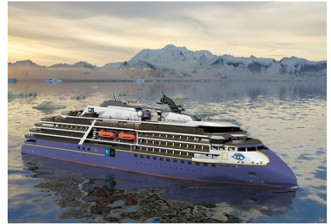
LINDBLAD EXPEDITIONS M.V. National Geographic Endurance 2 x GE 8L250MDC and 2 x 12V250MDC (Diesel Electric Power and Propulsion) Arctic Excursion Cruise Vessel
