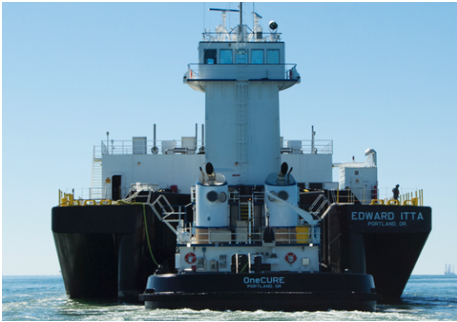
HARLEY MARINE M.V. Harley One Cure 2 x GE 6L250 Marine Engines (Mechanical Propulsion) Articulated Tug Barge (ATB)
